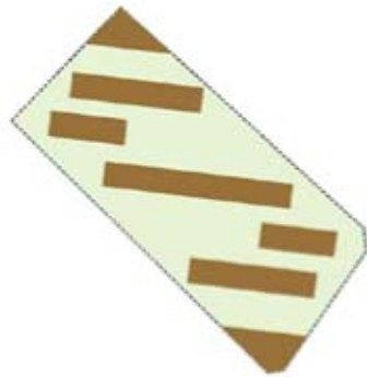
Benefiting from Existing Humidity Strips positioned to preserve existing water
